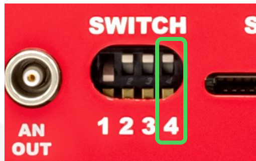
Figure 10: Saved Configuration at start-up
