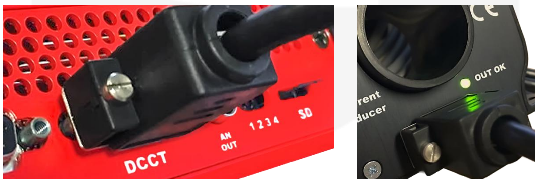
Figure 5: Connection of the DCCT cable
