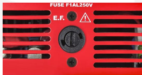
Figure 12: earth fuse housing
